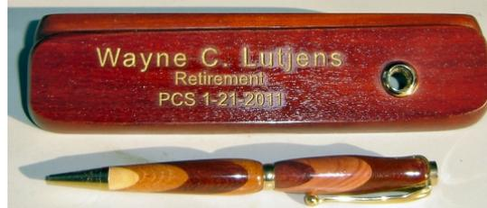
It is best to lightly coat the wood with a clear finish - so that the color fill can be wiped away from the un-engraved area and not fill in any wood grain.
